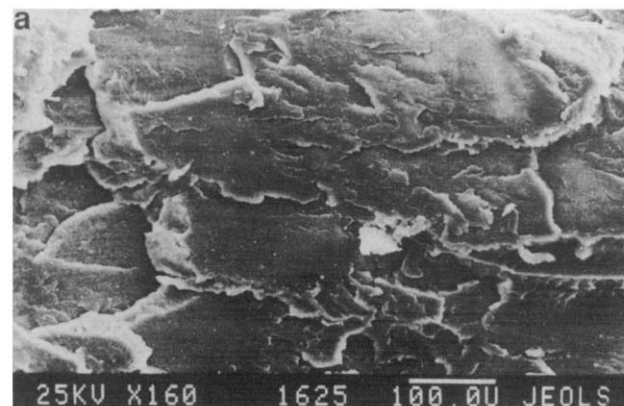
Figure 19 SEM micrograph of fracture surface of slowly drawn double-notched specimen obtained from precipitated ABS
