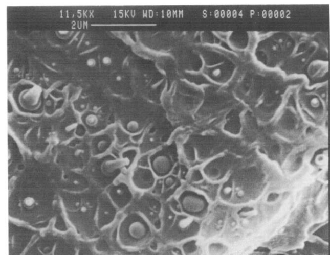
Figure 6 SEM micrograph of fracture surface 1 mm behind the notch of PS/PB/ABS blend: detail
